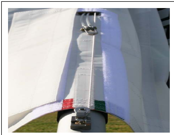
Figure 68 Section 4. De-tension Pull Back Cable
