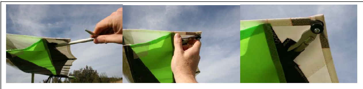
Figure 26 Section 4. Load Over-Centre Battens
