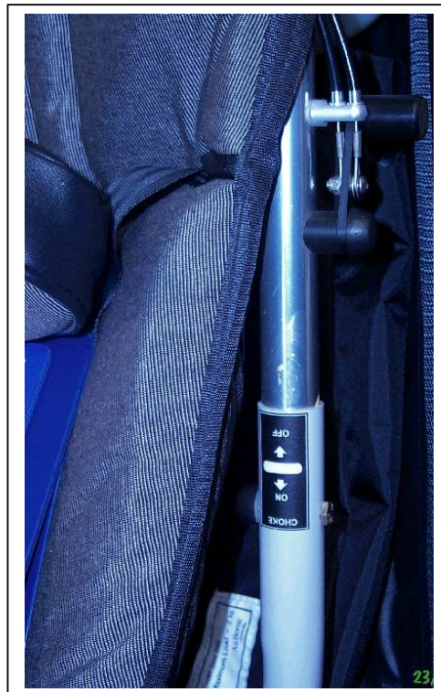
Figure 5 Section 2. Choke Placard Location (Under Seat Bag Placard in Background)
