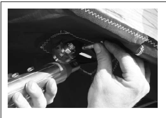
Figure 66 Section 4. Remove Strut to Leading Edge Connecting Bolt
