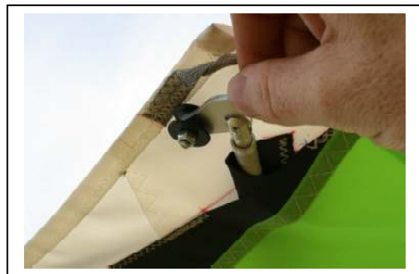
Figure 59 Section 4. Unload Over-Centre Tip Battens
