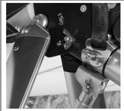
Figure 29 Section 4. Attach Wing to Wing U-Bracket
