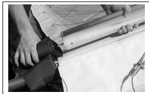
Figure 53 Section 4. Remove Kingpost
