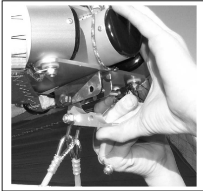
Figure 65 Section 4. Disconnect Nose Catch and Remove Nose Cone
