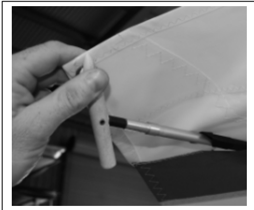
Figure 41 Section 4. Detension Tip Strut
