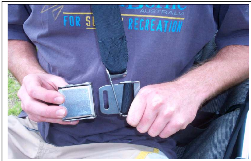
Figure 2 Section 7. Restraint harness, shoulder sash & buckle fitting.
