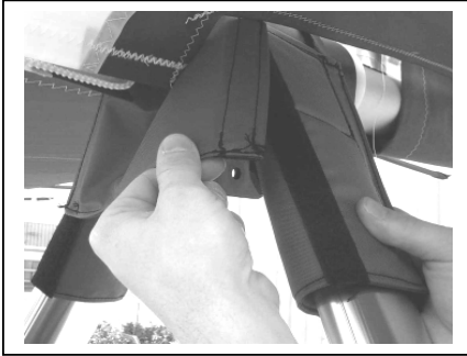
Figure 47 Section 4. Velcro U-Bracket Face Cover
