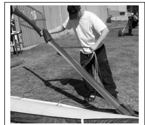
Figure 55 Section 4. Disconnect Base Bar
