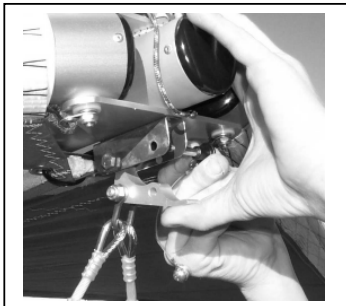
Figure 8 Section 4. Attach Nose Catch
