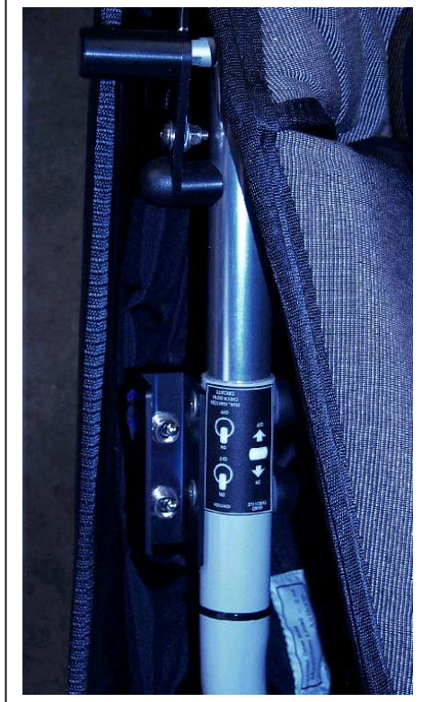
Figure 3 Section 2. Hand Throttle and Ignition Placard
