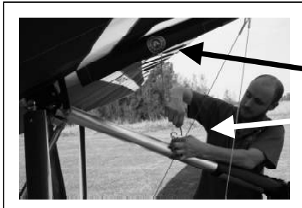
Figure 31 Section 4. Attach Trimmer to Mast
