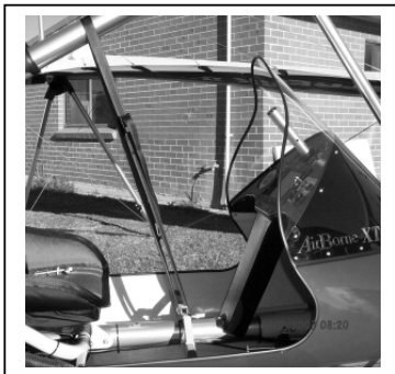
Figure 27 Section 4. Attach Mast Retaining Strap
